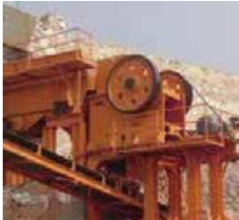
Mining and quarry fodder conveyor belt, crusher, lift
